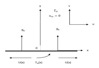
Figure 1 Flow Geometry
